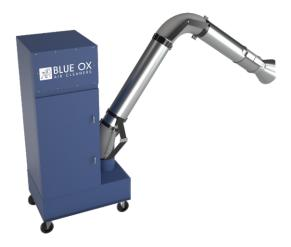
BLUE OX 1050P-DD has been designed for a high degree of mobility. Four large casters provide stability, while the units is being moved and a 'step-on' mechanism firmly looks the unit to the floor while it is in use. The pick-up arm is a full 8" and unlike most other units, has no internal support mechanism to obstruct the free flow of dirty air into the unit from the work area. External springs counterbalance the weight of the arm with friction joints added for complete stability.
