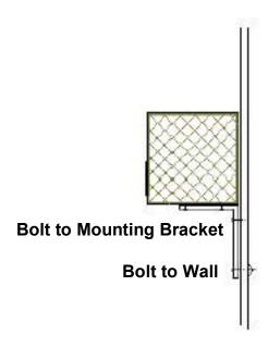
L-Brackets should be 6" from the ends of the unit
