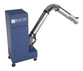
BLUE OX 1050P has been designed for a high degree of mobility. Four large casters provide stability, while the units is being moved and a 'step-on' mechanism firmly looks the unit to the floor while it is in use. The pick-up arm is a full 8" and unlike most other units, has no internal support mechanism to obstruct the free flow of dirty air into the unit from the work area. External springs counterbalance the weight of the arm with friction joints added for complete stability.
